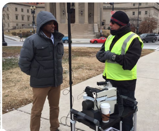
Trombino (right) demonstrates the RaFITS device with a high-purity germanium detector. (Photo: LLNL)
