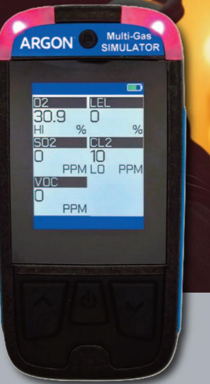
standard AA batteries, requires no calibration gases and can pair with an instructor's app via Bluetooth for real-time oversight. The aim is accurate, instrument-level simulation that reflects what frontline responders genuinely rely on.
