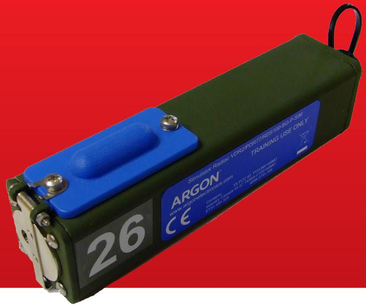
The DT616-SIM simulator probe set provides you with a training system that enables your students to experience the operational features of equivalent Canberra DT616/VDR-2 probe without the need to utilize real radiation sources or radioactive materials.
