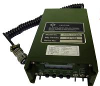
DT616-SIM can be used with AN/PDR-77 and RDS-100 radiation meters.
