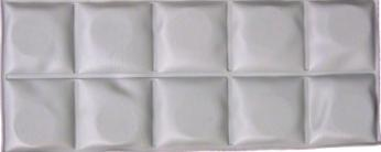
Simulation Beta source for contamination monitoring and decontamination training.
