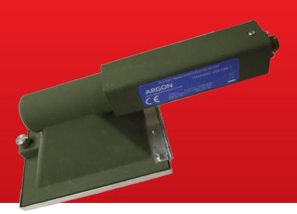
The A-SIM-P simulator probe set provides you with a training system that enables your students to experience the operational features of equivalent Canberra RDS-100 and AN/PDR-77 probe without the need to utilize real radiation sources or radioactive materials.
