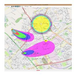
The HRM-SIM system is compatible with Argon's PlumeSIM system. PlumeSIM enables real time instrumented wide area operational training exercises to be conducted using single or multiple simulation device types that respond in the real world to multiple virtual radiation or chemical hazard release events.
