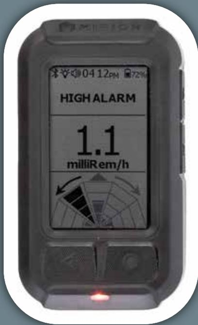
Radar mode indicating simulation source location.
