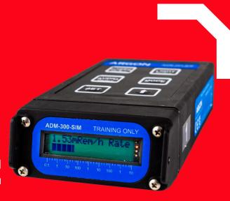
The ADM-300-SIM survey meter simulator enables your students to experience every operational feature of the real Mirion/Canberra ADM-300A (V1B) without the need to utilize an ionizing gamma or beta radiation source.
